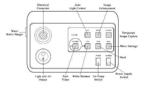
Electrical Connector: This is the socket that connects to the electrical pins on the light guide connector of the endoscope.
